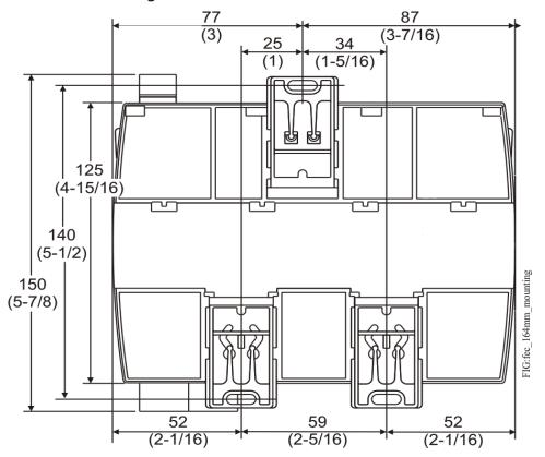
Figure 2: Back of PCA2513 Controller
