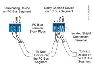
Figure 4: FC bus terminal block wiring
