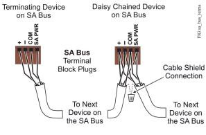
Stranded, 4-Wire (2 Twisted Pair) Shielded Cable (One twisted pair is the + and - leads.
